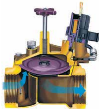
EFB-CP Cutaway
